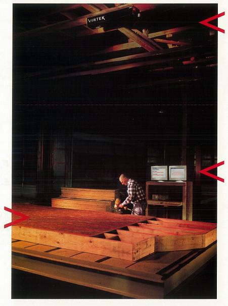
Project templates up to 14' x 14'. Unlimited panel size can be achieved using multiple laser projectors.
